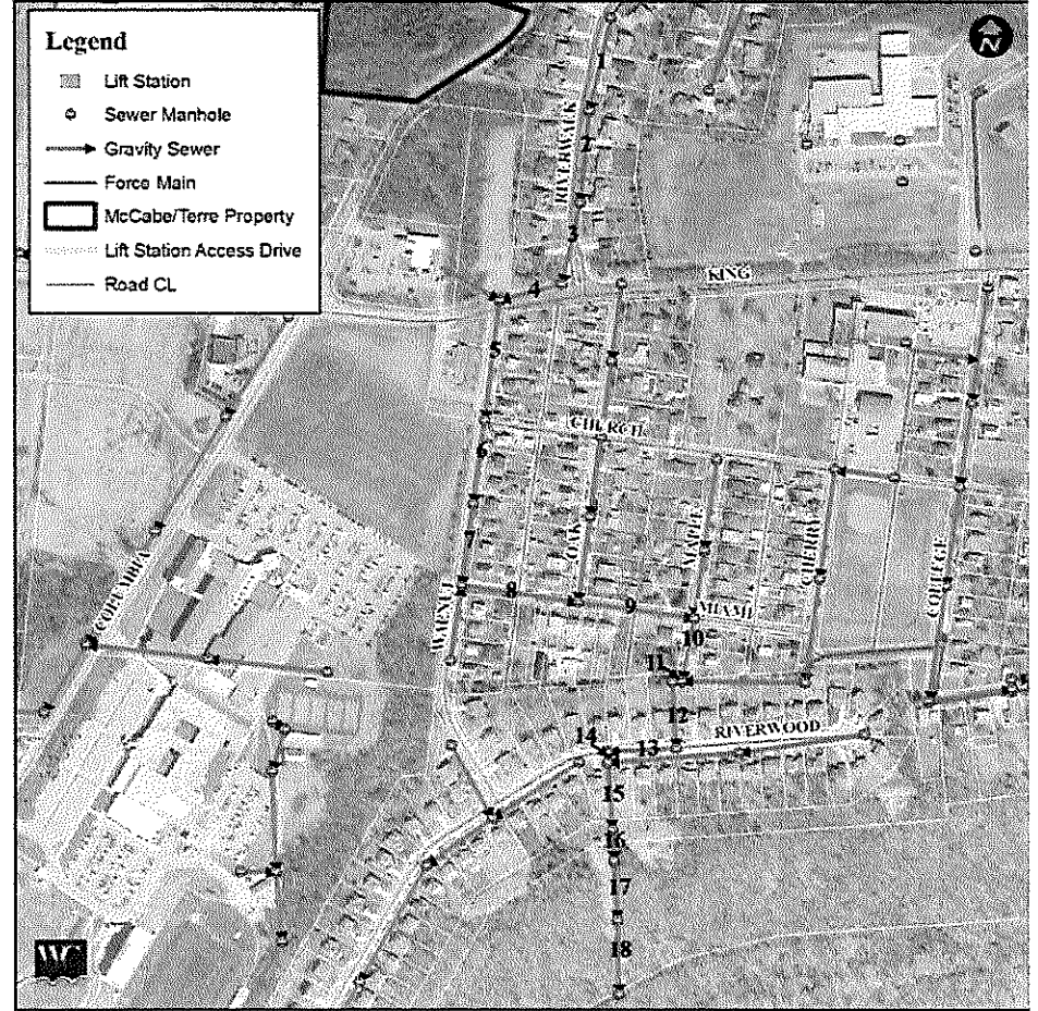
Gravity Sewer Sections (after existing Force Main)
