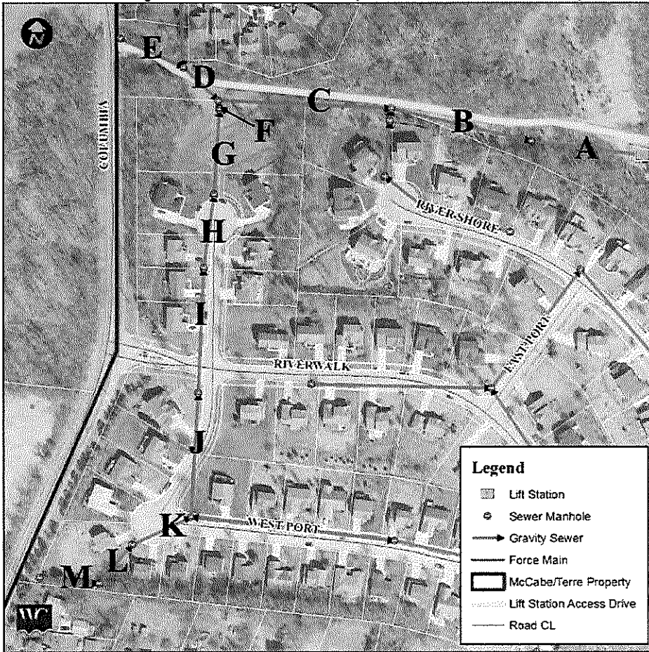
Gravity Sewer Sections (before Lift Station)
